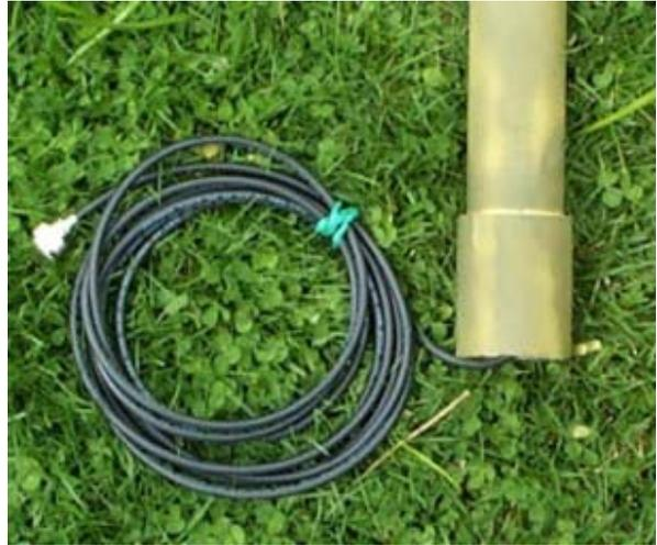
Install pipe coupling to one end of the pipe as seen above. Install a coupling to the remaining pipe as well. The couplings need not be glued... in fact I didn't glue any of the caps or couplings and they seem plenty sturdy for the purposes of the support mast.
