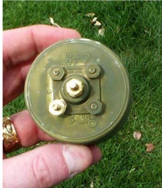
Cut off the head of a 1" #6 brass screw and solder it in the center post of SO-239.
